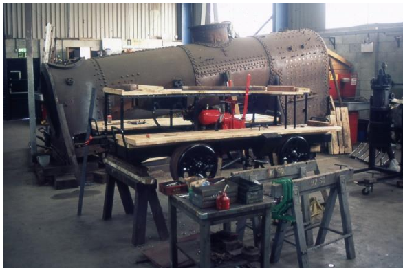
Inside the Heavy Overhaul Shed. A pre-overhaul 656 boiler forms a backdrop to the under-overhaul Wickham Trolley.
